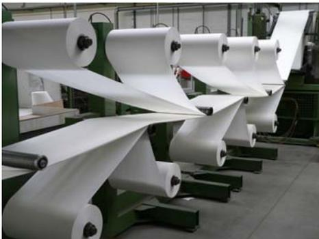
Reel unwind equipment for round filter production
